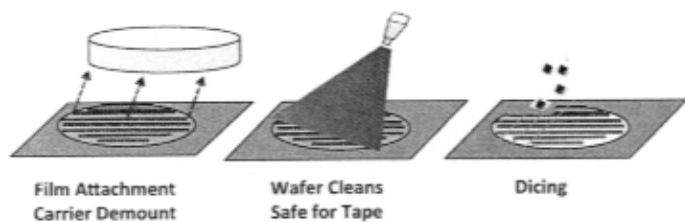
Fig. 8. Process flow for cleans while product wafer is supported on tape (film frame).
