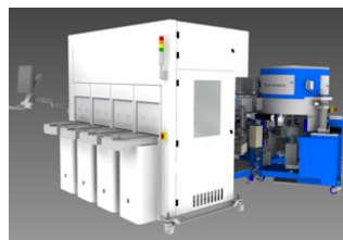
Fig. 16: Vacuum process configuration testing using a PVD system designed for EMI shielding. [2]
