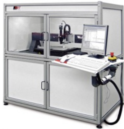
MicroProf® 300 Multi Sensor metrology tool with 300 mm stage and optional housing
